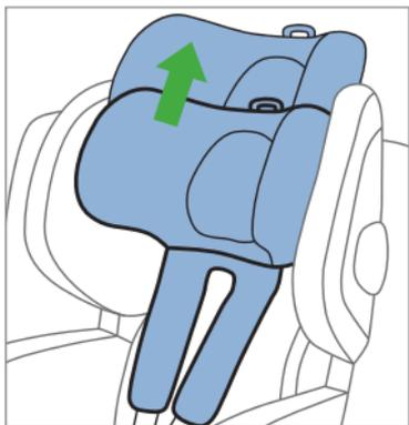
Now move the headrest into the required position and let the locking mechanism lock in place.
